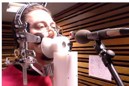
Figure 1: The participant speaking into the EVA mask while wearing the UTI headset.
